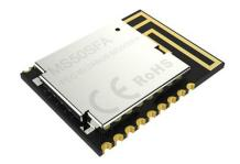
MS50SFA is a compact (15.8 x 12.0 x 2.0 mm), highly flexible, ultra-low power wireless BLE 5.0 Module based on nRF52810 SoCs; Its powerful 32-bit ARM Cortex<sup>™</sup> M4 CPU, a 192KB Flash memory, a 24KB RAM and integrating a 2.4 GHz transceiver can offer the perfect solution for Bluetooth connectivity.
