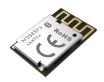
MS88SF3 is advanced, compact (18.5mm  $\times$  12.5mm  $\times$  2mm), highly flexible, ultra-low power wireless BLE 5.0 Module based on nRF52840 SoCs. Its powerful 32-bit ARM Cortex<sup>TM</sup> M4 CPU, a 1 MB flash memory, a 256KB RAM and integrating a 2.4 GHz transceiver offers the perfect solution for Bluetooth connectivity.
