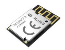
MS88SF3 is advanced, compact (18.5mm  $\times$  12.5mm  $\times$  2mm), highly flexible, ultra-low power wireless BLE 5.1 Module based on nRF52833 SoCs. Its powerful 32-bit ARM Cortex<sup>TM</sup> M4 CPU, a 512KB flash memory, a 128KB RAM and integrating a 2.4 GHz transceiver offers the perfect solution for Bluetooth connectivity.
